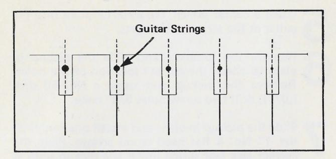
Bend the template so that the slotted portion is perpendicular to the guitar body and push it flush with the bridge. Tape the ends of the template in place.
