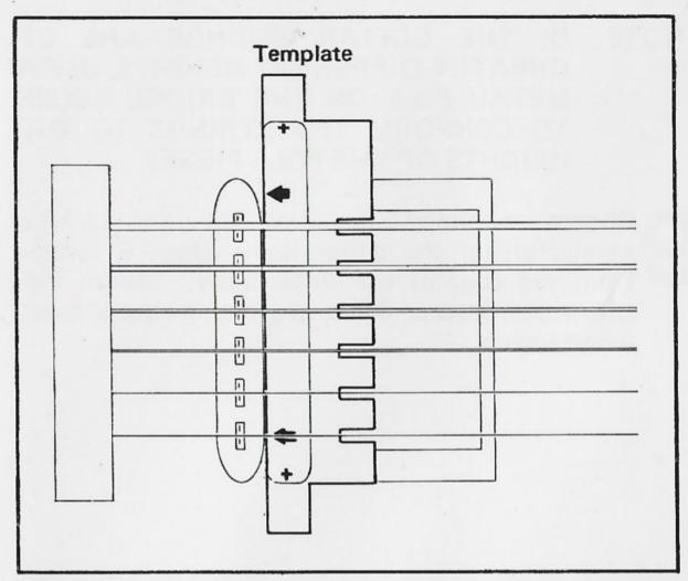
3 Center as many of the strings in their respective slots as will fit. Do not bend the template. If any of the strings do not fit the template, replace or refile the bridge shoes so that all strings are centered in the slots. For best performance, the strings must be centered in the slots.
